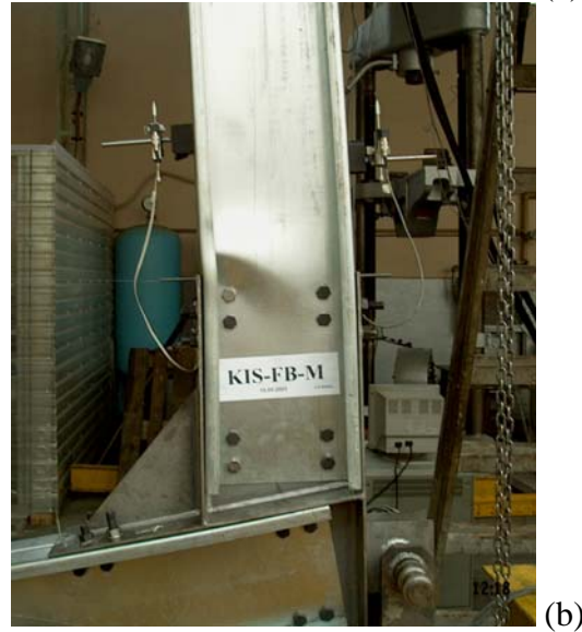
Figure 5. Failure of knee specimens KIS-M (a) and KIS-FB-M (b).
