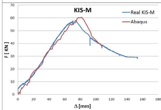
Figure 8. Knee and ridge specimens:  $F-\Delta$  experimental and numerical curves
