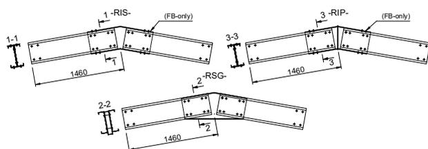
Figure 1. Configurations of ridge joints.
