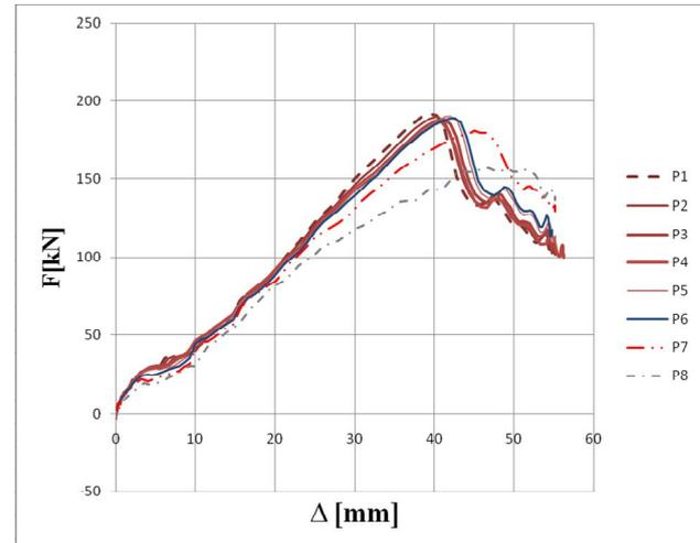
Force – displacement graphs, ridge specimens RIS-FB-M with flange bolts
