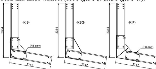
Figure 2: Configurations of knee joints
