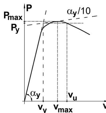
Figure 10. ECCS procedure to define the yield displacement
