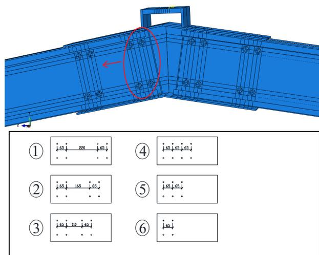
Figure 9. RIS-M ridge specimens used in parametric study
