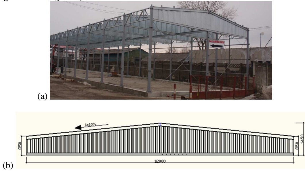
Fig. 1: (a) Structural solution; (b) Geometry of the proposed specimen for testing
