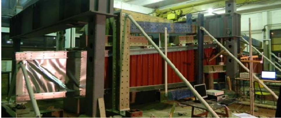
Fig. 8: Deformed shape of Beam-1 at failure
