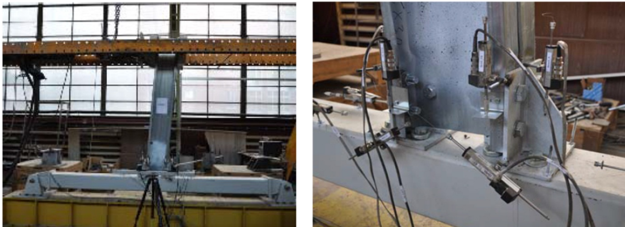
Fig. 14 – HBBC connection – monotonic test.
