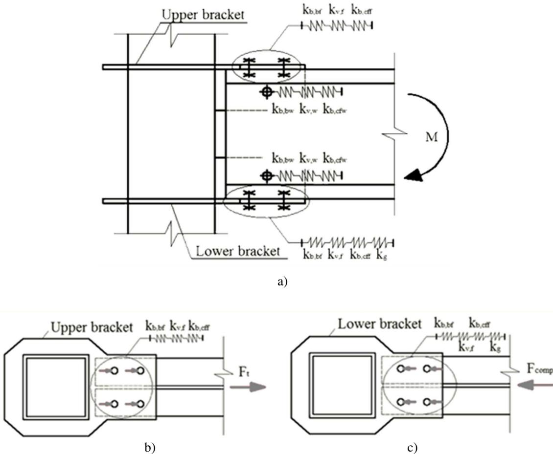
Figure 6: Identified components: a) side view, b) upper view, c) lower view.
