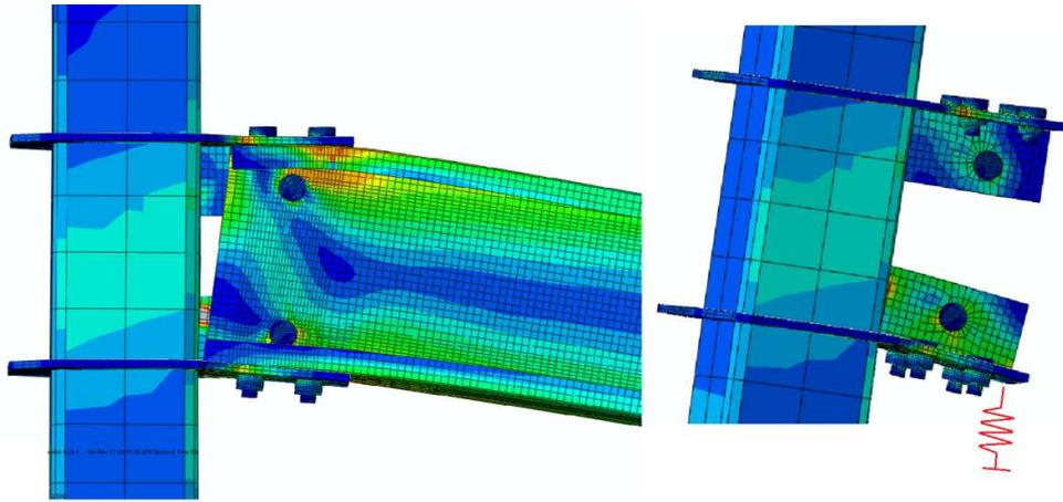
Figure 3: FEM detail with deformation of the lower bracket.
