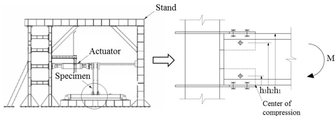
Figure 2: Experimental test setup and DCBC joint model geometry.
