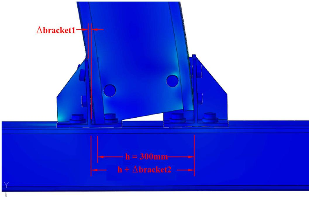
Figure 15: Deformations (20x) due to the shear in the hollo-bolt connection (at elastic region).
