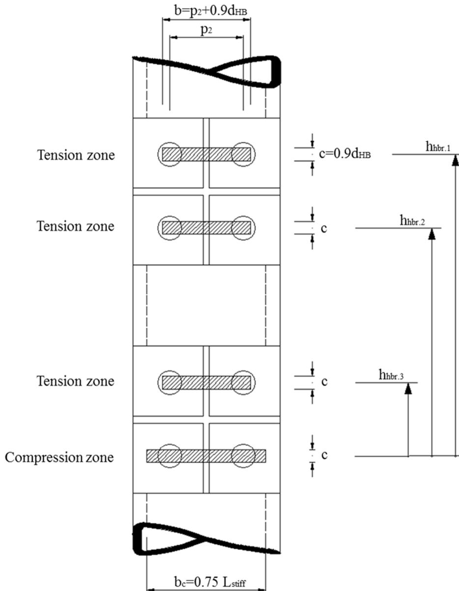
Figure 12: HBBC joint geometry with SHS face tension/compression zone similarly to Weynand *et al.* method [17].
