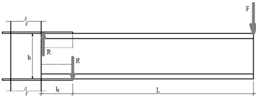
Figure 4: Geometrical details of the tested specimen.
