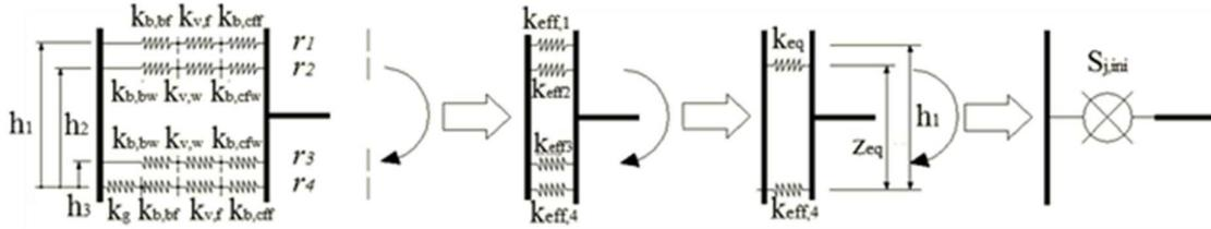
Figure 7: Proposed mechanical model and procedure for evaluating the rotational stiffness.
