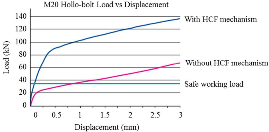
Figure 13: M20 Hollo bolt performance according to Lindapter [18].
