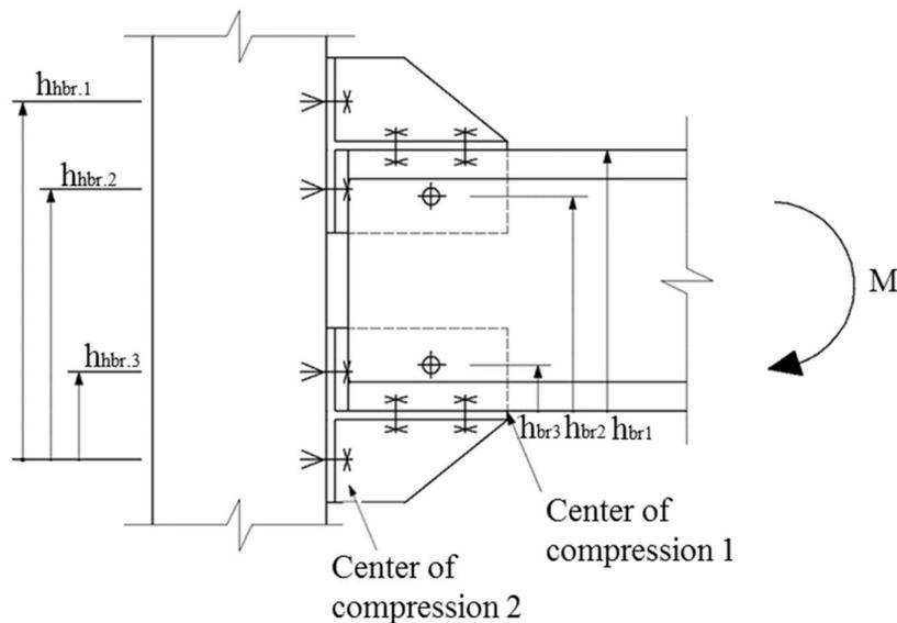
Figure 9: HBBC joint model geometry.
