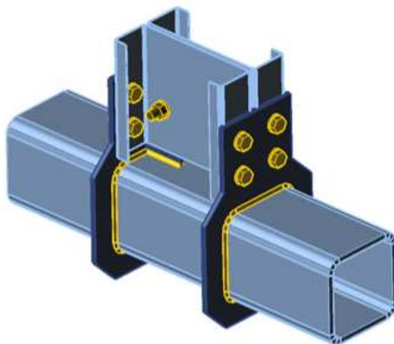
Figure 1: DCBC connection configuration.
