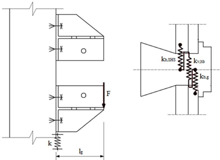
Figure 14: Components considered active in the displacement of the lower gusset due to the shear in the hollo bolt connections.
