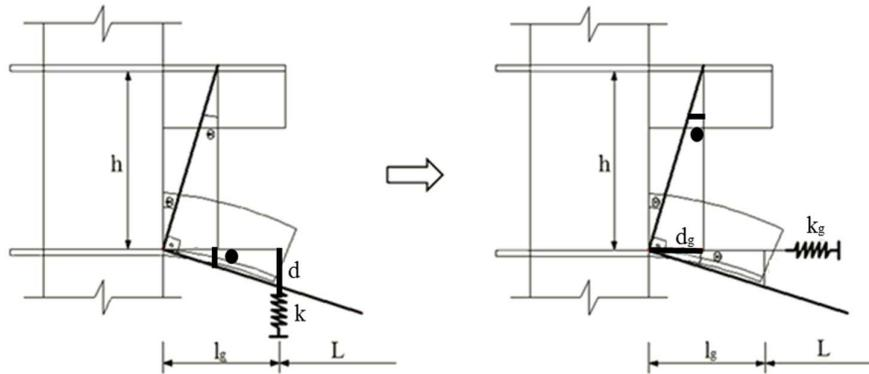
Figure 5: Component lower bracket in bending.
